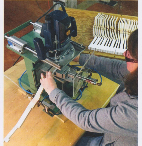
April Larson uses a precision industrial router to square the key fronts.
