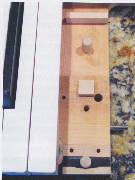
Accessory cheek blocks are precisely doweled to the keyframe, secured by a single flat-head wood screw from the underside of the frame.
