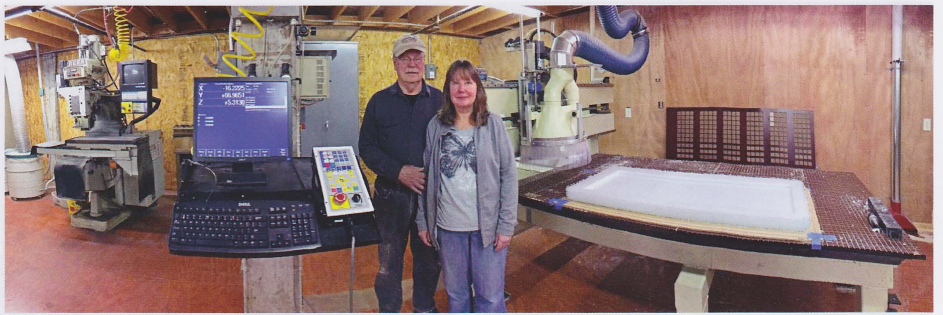
Bob and April Larson. Two computerized machines make most of the parts. The milling machine (left) makes all the metal parts for the actions. Bob built the router shown behind April's left shoulder. Note the cutout of the foam shipping insert on the work table.
